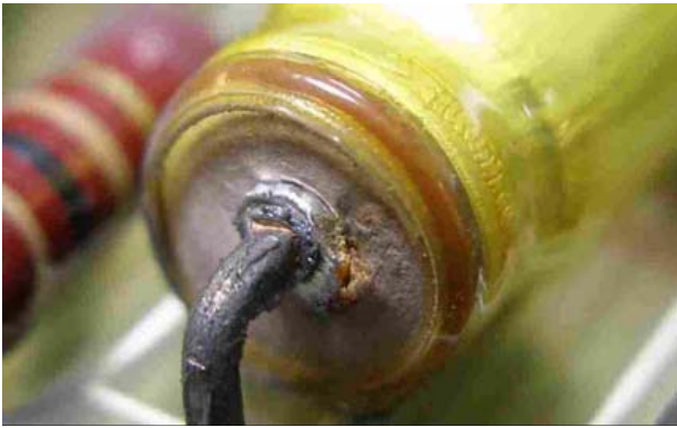
Fig. 4: Damaged chemical capacitor shown in figure 1 of paper 299
