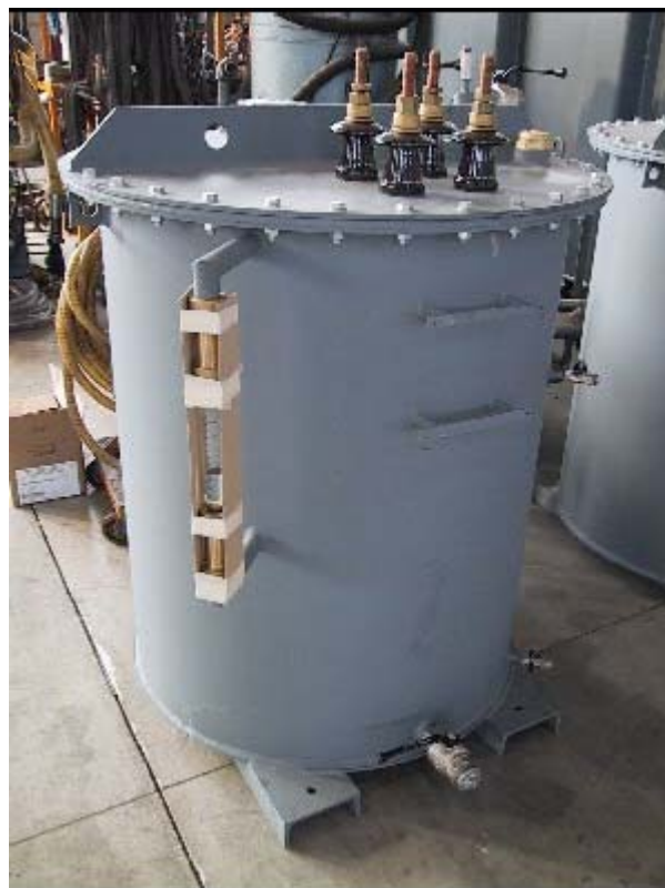
Fig. 9: Single phase device for thermal ageing shown in Figure 1 of paper 555
